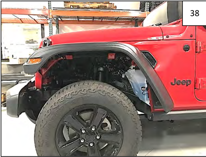
Complete Front Flare installation.
