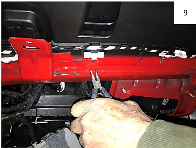
Disengage 9 white factory brackets that are holding factory flare onto vehicle, spaced along wheel well. All but 1 bracket are accessible by pliers. If you wish to preserve the paint finish (which will be covered by flare), use a plastic pry tool to help remove retainers.
