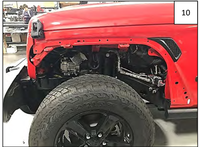
Pull factory flare from vehicle. Pry any white retainers from sheet metal and discard – holes must be clear for installation. Retain factory flare to remove light housing in next steps.
