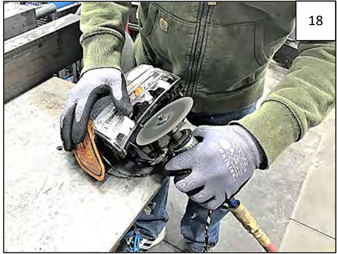
Using a cutoff wheel or saw, cut 4 plastic tabs on light housing as shown.
