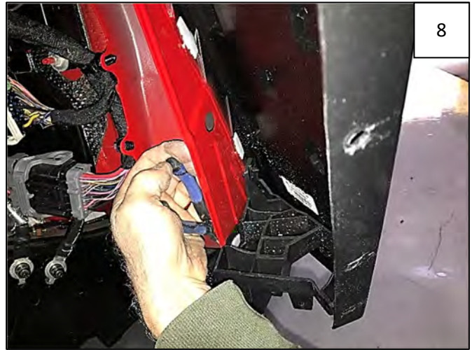
To remove lower bracket, use pliers behind bracket and sheet metal to disengage 2 white factory retainers. Discard.
