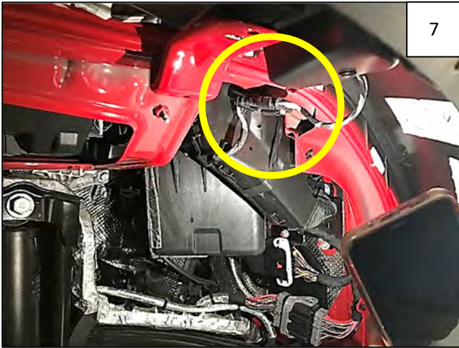
Disconnect Light Wire Harness by pushing the red tab out to unlock. Push the release tab and pull the harness out.
