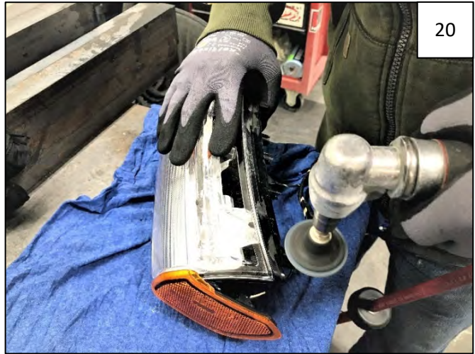
Using a sanding disc or sandpaper, sand down any remaining tab vestiges. Tab vestiges must be as flush as possible for proper installation.
